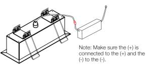
Turn off the power supply and connect the wires from the remote driver to the wires of the luminaire by the means of the connector.
