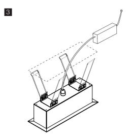
Lift the springs up and insert the luminaire into the cut out.
