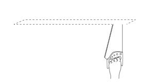
Make a cut out in the surface of the dimensions 15cm: 50 x 172 mm 30cm: 50 x 327 mm.
